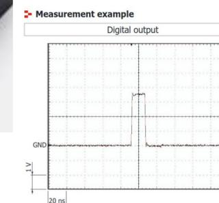
TTL-compatible digital output pulse
