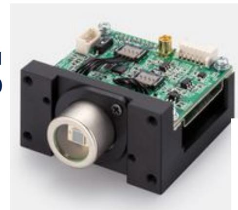
3 mm<sup>2</sup> photosensitive area, peak sensitivity 450 nm
