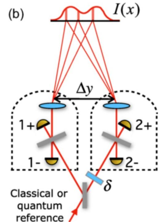
Demonstrating table-top interferometric imaging using a path-entangled single photon towards quantum telescopy (Brown et al. PRL 2023)
