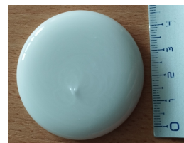
Alumino-Silicate glass: the white color is due to phase separation.
